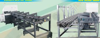
Automatic material feeding via an inclined loading magazine allows unmanned sawing operation even for material lengths in excess of 6 m with stacking area for raw material up to 800 mm (Above FANC 100) model. This Loader works on Cam mechanism which helps the bar smoothly loaded on the machine without any impact. This supported detection of the work piece starting point for trim cutting.
