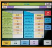
The data for cutting lengths and numbers can be easily entered step-by step via user friendly colour "touch screen" display with graphics. Easy for feeding the required data and monitoring of cutting in single screen. User friendly operating module includes self diagnostic function on-screen for Trouble shooting, with an automatic detector for any malfunction the screen will show an Alarm, so that the problem can be easily identified and resolved
